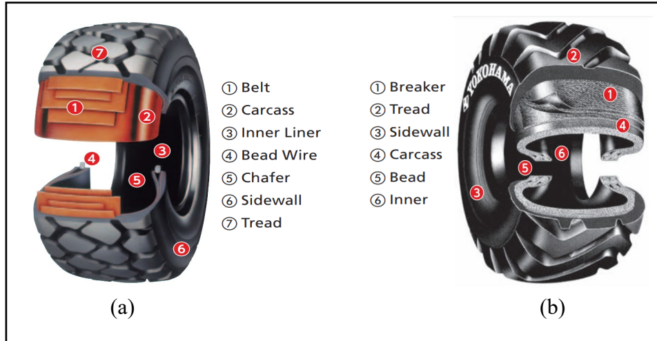
Figure 2.3 Structural Diagram of Radial Tire (a) and Bias Tire (b) (Yokohama Rubber Co., 2021)
